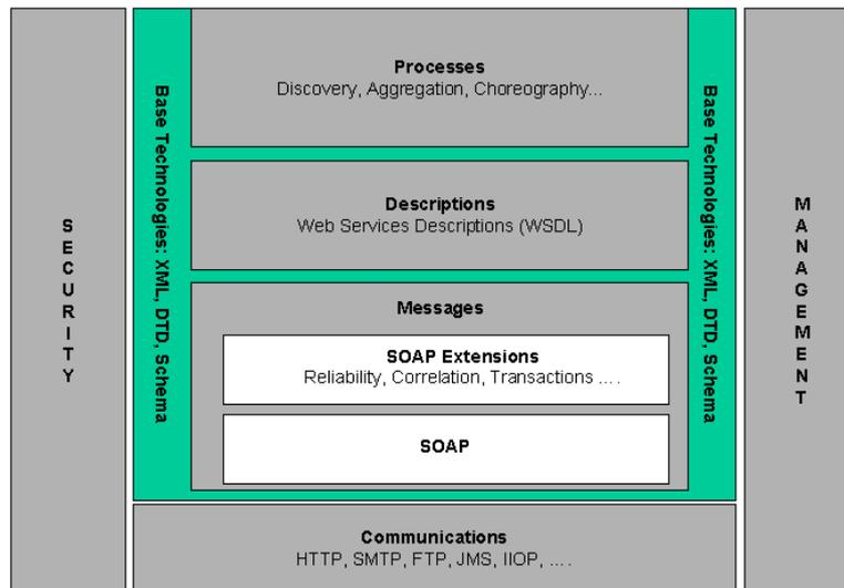
**Figure 4: W3C Web Service Architecture Stack**
